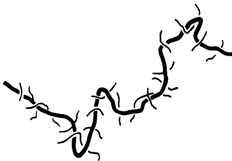
FIG. 21. Sketch showing one entire molecule together with the segments of other molecules that are located near to it and restrict its motion (from Dealy and Wissbrun, 1990).
